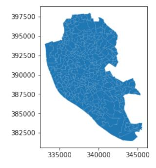
Although in some contexts this may be desirable (or at least, accepted), in many it will not. From a cartographic point of view, maps need to be as good representatios of reality as they can. We can ensure the scaling ratio between both axes remains fixed, whichever the shape of the figure. To do this, we only need to add a single extra line of code: plt.axis("equal").
