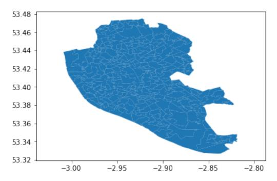
Because the area we are visualizing is not very large, the shape of the polygons is roughly the same. However, note how the *scale* in which they are plotted differs: while before we had coordinate points ranging 332,000 to 398,000, now these are expressed in degrees, and range from -3.05 to -2,80 on the longitude, and between 53.32 and 53.48 on the latitude.
